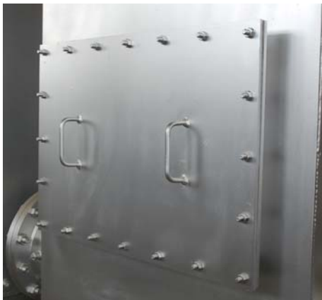
Fig. 7: Discharge gate with bolted cover
